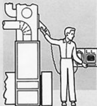
Furnace interior inspection.
